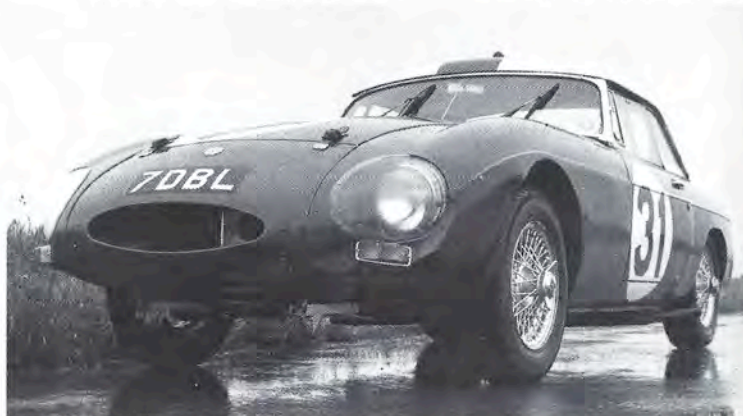
The MGB raced in 1963. To garner a higher top speed, it sported a fibreglass hardtop and a reshaped 'droop-snout' front, crafted in aluminium, complete with Perspex headlight covers
