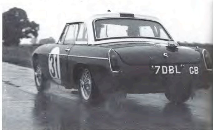
The MGB raced in 1963. To garner a higher top speed, it sported a fibreglass hardtop and a reshaped 'droop-snout' front, crafted in aluminium, complete with Perspex headlight covers
