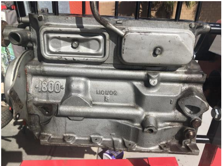
5 MAIN BEARING MGB SHORT BLOCK AVAILABLE 8GK-WE-H 1375
